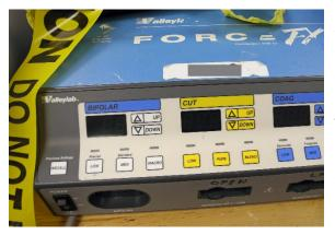
The electrosurgical unit (ESU) is a workhorse for surgical procedures. It uses high-frequency electrical current for cutting and coagulating tissue. There are also specialized ESU-type devices, including those that incorporate argon beam and ultrasonic vibration technologies.
